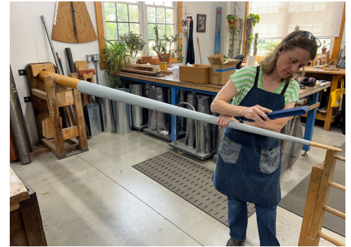
Shaping one of the pipes by hand.
