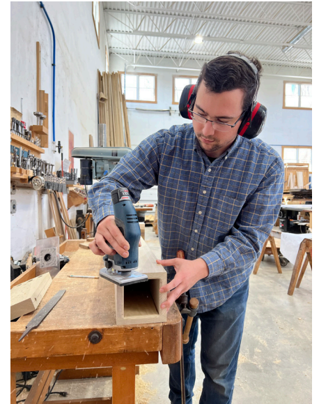
Sanding down one of the wooden pipes.
