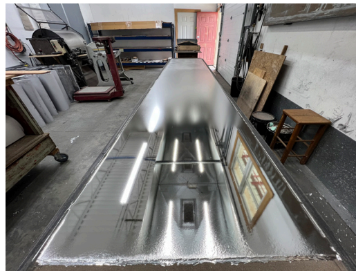
Metal for pipes just poured onto table, preparing for cooling and cutting
